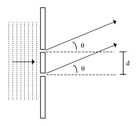
• By "idealized" double slit experiment, we assume that the Huygens' waves radiating out from each slit and reaching a point on the distant screen are just circular waves of the form
